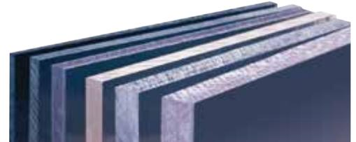
**Exolon® AR** sheet is an abrasion and enhanced UV resistant polycarbonate sheet that offers glasslike hardness coupled with the impact strength of standard polycarbonate. Additionally, **Exolon® AR 8099** offers on both surfaces enhanced resistance against yellowing and hazing for an extended service life in high profile architectural glazing. **Exolon® AR 7099** is a one sided hardcoated sheet which can be used for lamination and printing on the uncoated side.
