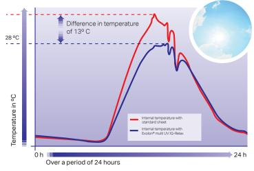
Real-life tests in unventilated conservatories have proven a remarkable heat reduction up to 13°C compared with standard opal sheets. This means an excellent result that guarantees a pleasant room temperature independent of the weather. The extraordinary homogeneous gain in light results in a comfortable "light ambience".
