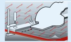
**6** | Marking should be done with a soft crayon on the masking film, which should be left on the sheet during machining and until the sheet has been installed. For cutting, use conventional circular saws with unset, multi-tooth carbide-tipped blades. Always work with a stop.
