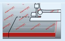
**9** | Corner cutouts are often required (e.g. for pipes, ventilation etc.). Use a jig saw without pendulum action. Drilling can be performed with twist drills (point angle φ 110°-130°), conical or step drills.
