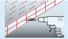
**7** | Swarf that has entered the sheet chambers can be blown out with compressed air or removed using a vacuum cleaner.
