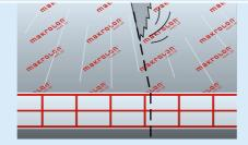
**8** | If the sheet width of Makrolon® multi UV sheets has to be reduced, please cut as close as possible to the next web to ensure the best clamping action of the glazing bar.
