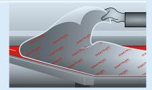
**13** | Finally, remove the masking film from the Makrolon® multi UV sheets. It should not be exposed to weathering for more than 24 hours.
